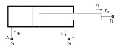
For example, the model of a double-acting hydraulic cylinder shown in the previous illustration can be described with a simple set of equations:
