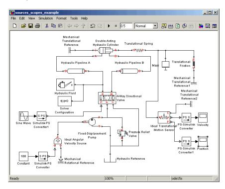
The system in the diagram consists of a double-acting hydraulic cylinder controlled by a 4-way directional valve. The valve is driven by a Simulink signal, which is first converted into a Physical Signal with the Simulink-PS Converter block (named Simulink-PS Converter1 in this diagram) and then fed to the valve control port S. The power unit of the system is built
