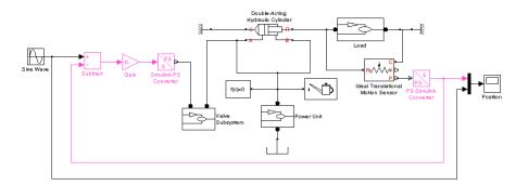
A better way to avoid an algebraic loop without introducing additional dynamics is shown in the modified model below.
